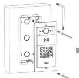
Use two M4x15 Torx Screws to lock the device's straight wall side.
